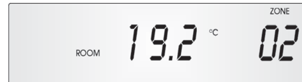
Figure - Check Temp (Multi-zone)
